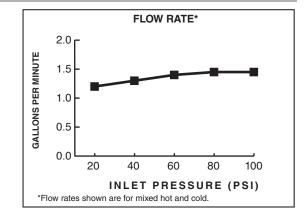
1.5 gpm/5.7 L/min. FLOW RATE
