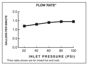
1.5 gpm/5.7 L/min. FLOW RATE
