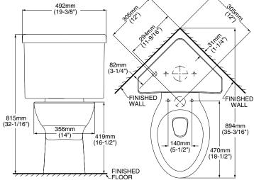
THIS TOILET IS DESIGNED TO ROUGH-IN AT A MINIMUM DIMENSION OF 305MM (12") FROM FINISHED WALL TO C/L OF OUTLET. SUPPLY NOT INCLUDED WITH FIXTURE AND MUST BE ORDERED SEPARATELY. \* DIMENSION SHOWN FOR LOCATION OF SUPPLY IS SUGGESTED.
