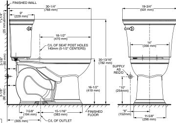
THIS COMBINATION IS DESIGNED TO ROUGH-IN AT A MINIMUM DIMENSION OF 305MM (12") FROM FINISHED WALL TO C/L OF OUTLET. \* DIMENSIONS SHOWN FOR LOCATION OF SUPPLY ARE SUGGESTED. SUPPLY NOT INCLUDED WITH FIXTURE AND MUST BE ORDERED SEPARATELY.
