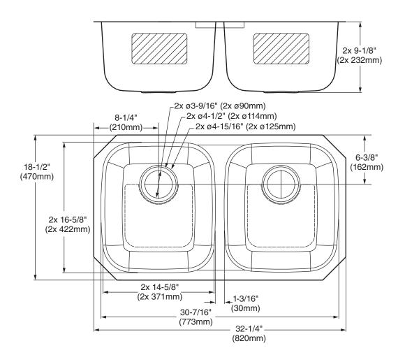
**NOTES:**\* DIMENSIONS SHOWN FOR LOCATION OF SUPPLIED AND "P" TRAP ARE SUGGESTED. FITTINGS NOT INCLUDED WITH FIXTURE AND MUST BE ORDERED SEPARATELY. SEALING COMPOUND SUPPLIED BY OTHERS.
