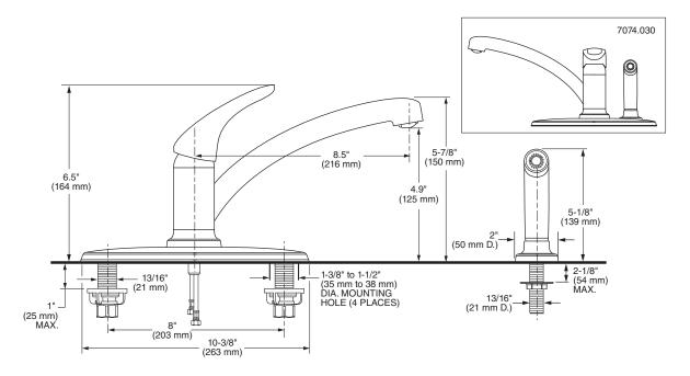
NOTES: \* DIMENSIONS SHOWN FOR LOCATION OF SUPPLIED AND "P" TRAP ARE SUGGESTED. SEALING COMPOUND SUPPLIED BY OTHERS.
