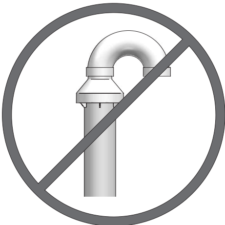
Figure 5-5 Do Not Install U-Bend to Rain Cap
