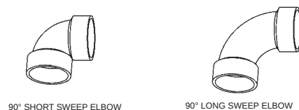
Figure 23. Vent Pipe Elbows
