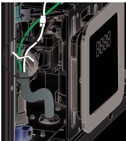
Figure 40 - System power cord cut location.
