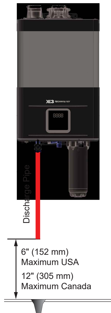
Figure 38 - Discharge Pipe Clearance
