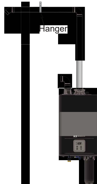
Figure 21 - Power Vent Horizontal Installation
