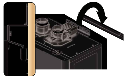
Figure 6 - Use Mounting Screws to Secure Water Heater to Bracket
