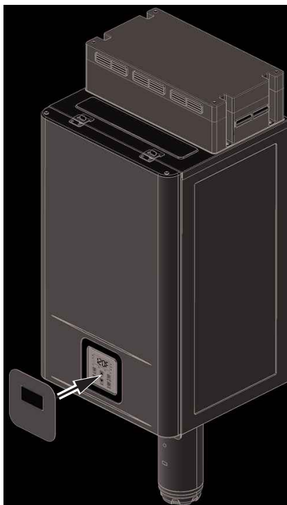
Figure 28 - Control Panel Cover Plate Install.
