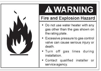
Make sure the gas supplied is the same type listed on the model rating plate. The inlet gas pressure must not exceed 14 inch water column (3.5 kPa) for natural and propane gas (L.P.). The
