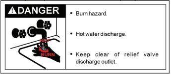
THE WATER PASSING OUT OF THE VALVE DURING THIS CHECKING OPERATION MAY BE EXTREMELY HOT. AVOID CONTACT AND DISCHARGE SAFELY TO PREVENT WATER DAMAGE.
