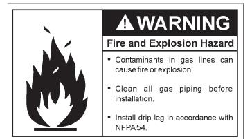
A drip leg (sediment trap) shall be installed as close to the inlet of the water heater as practical at the time of water heater installation. The sediment trap shall be either a tee fitting with a capped nipple in the bottom outlet or other device recognized as an effective sediment trap. If a tee fitting is used, it shall be installed in conformance with one of the methods of installation shown in Figures 8 and 9.
