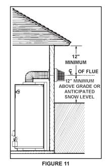
Be sure venting is properly connected to prevent escape of dangerous flue gases which could cause deadly asphyxiation.
