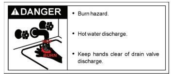
The temperature-pressure relief valve must be manually operated at least once a year. Caution should be taken to ensure that (1) no one is in front of or around the outlet of the temperaturepressure relief valve discharge line, and (2) the water manually discharged will not cause any bodily injury or property damage because the water may be extremely hot.
