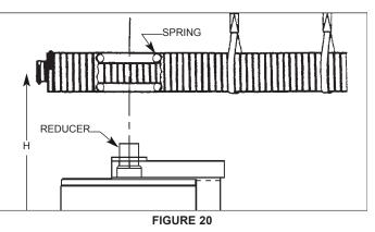
Bend both the corrugated tubes toward the water heater's flue connection.
