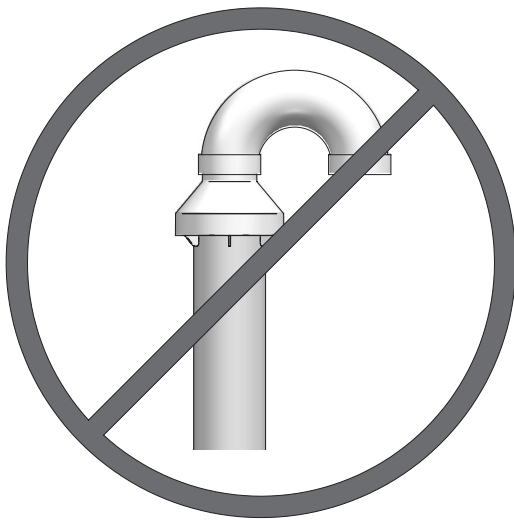
Figure 48. Do Not Install U-Bend to Rain Cap
