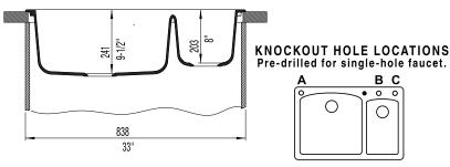
Note: Distance between B & C holes is approx. 5" on center, because of clip location.
