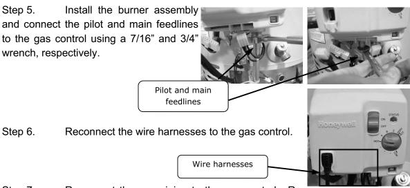
Step 7. Reconnect the gas piping to the gas control. Restore the gas supply and check for gas leaks.
