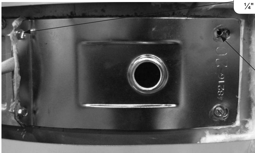
Verify threaded hole alignment with slotted openings in inner door.
