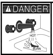
Water temperature over 125°F can cause severe burns instantly or death from scalds.
