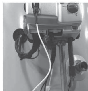
PRESSURE TAP SHOWN INSTALLED
