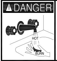
Water temperature over 125°F (52°C) can cause severe burns instantly or death from scalds.
