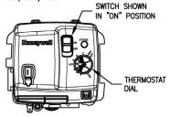
Slide the switch on the right side of the gas valve down to the "OFF" position
