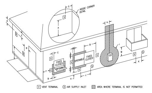
Figure 1 - Vent Terminal Clearances
