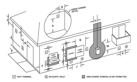
Figure 1 – Direct Vent Terminal Clearances
