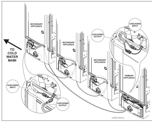
Fig. 2 Example of installation for: RTG 199HE, RTG 199ME
