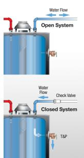
But today's plumbing regulations require the integration of backflow preventers or check valves, primarily to keep the water in your home from the possibility of contaminating the water supply. As a result, present-day hot water systems are considered "closed" systems.
