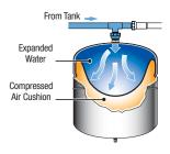
thermal expansion of water creates excess pressure within the water heater, excess water is forced into the expansion tank, keeping pressure levels within the normal operating range of the water heater.
