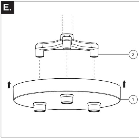
**E.** Place the escutcheon (1) over the manifold (2), aligning the escutcheon openings to the manifold outlets.
