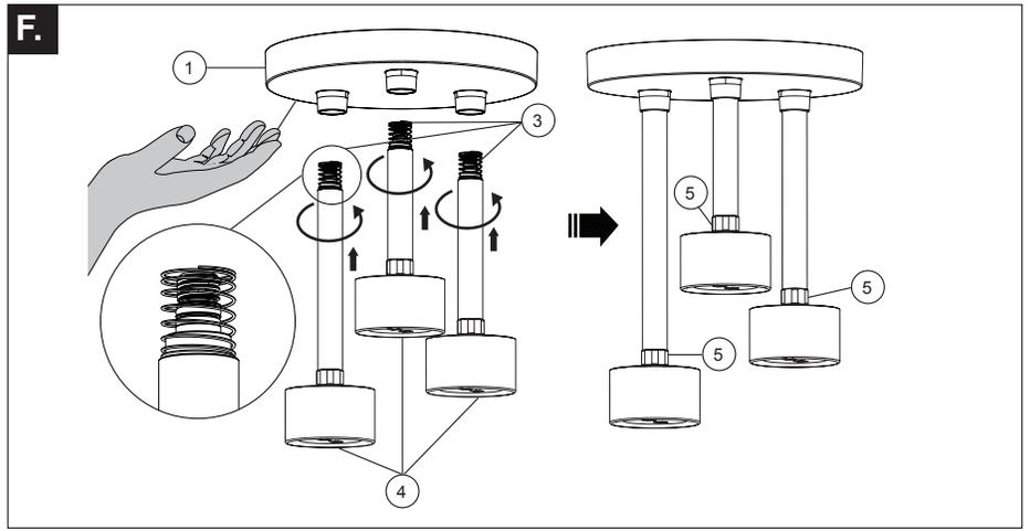
**F.** Ensure the springs (3) are located on the tube assemblies before assembling. Hold the escutcheon (1) in place by hand, assemble and hand-tighten each tube assemblies (4) to the manifold. Once all three tube assemblies are hand tightened and the escutcheon held in place, tighten each of the three tube assemblies an additional 1/4-turn more. **CAUTION: OVERTIGHTENING CAN RESULT IN DAMAGE!**
