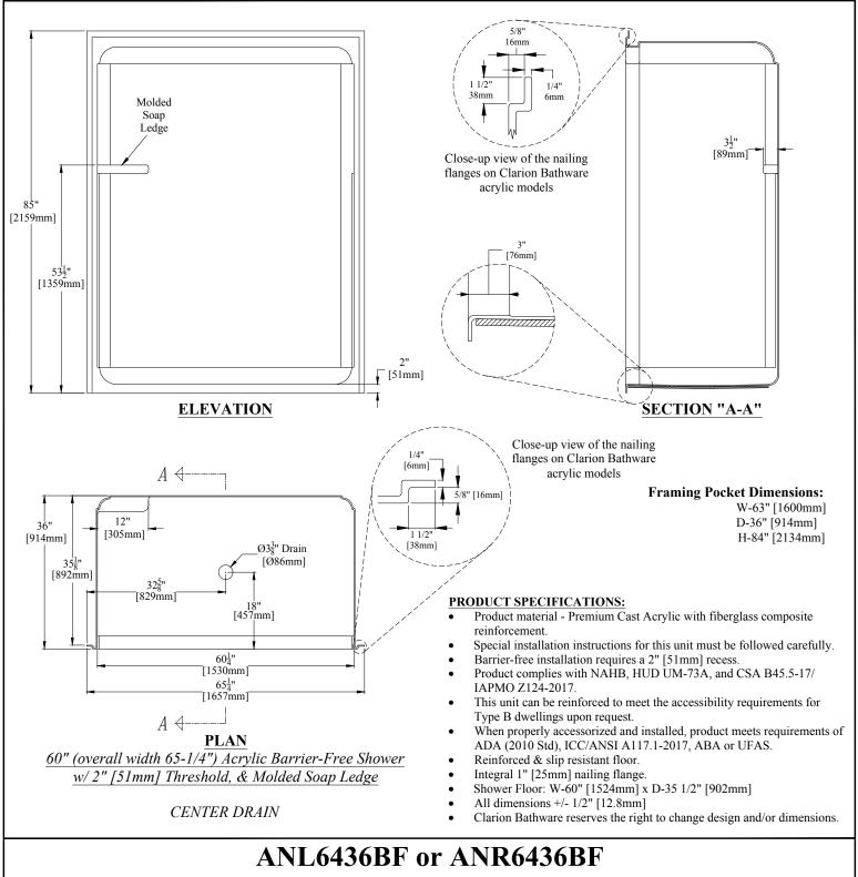
60" (overall width 65-1/4") Acrylic Barrier-Free Shower w/ 2" [51mm] Threshold, Molded Soap Ledge, Molded Dome, & Center Drain
