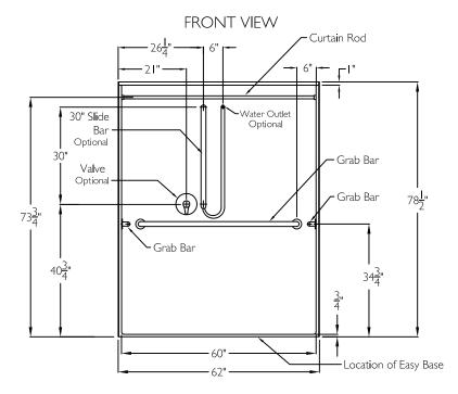
NOTE: Valve package may be located on the back wall or either end wall.
