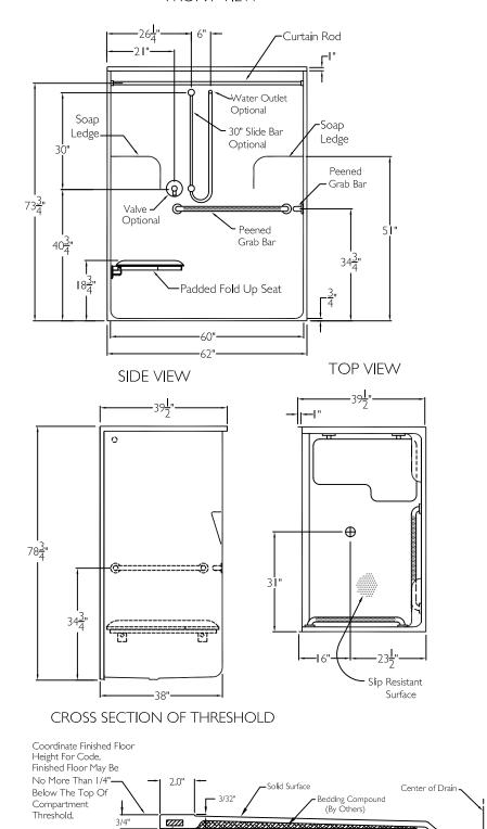
Drain Core 6" Minimum, Plus 1/2" Deep x 10" Dia. Recess
