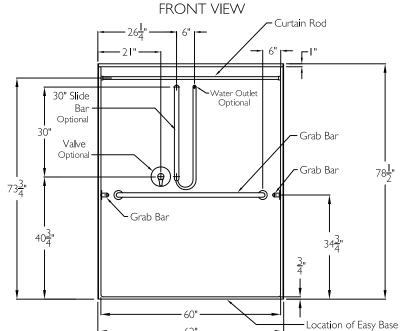
NOTE: Valve package may be located on the back wall or either end wall.
