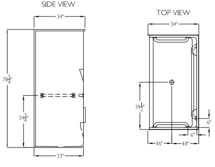
DRAIN CUT-OUT SIZE 10" DIA. x 1/2" DEEP RECESS, PLUS 6" DRAIN CORE.
