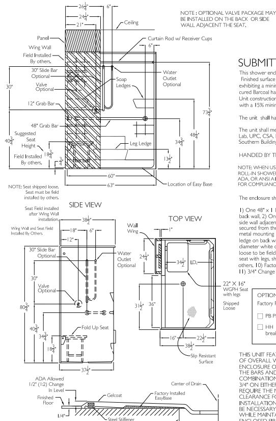
Drain Core: 6" Minimum Plus 1/2" Deep x 10" Dia. Recess.
