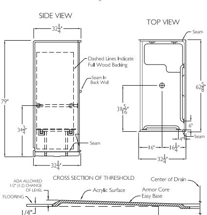
Drain Core: 6" Min. Plus 1/2" Deep X 10" Dia. Recess.
