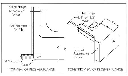
THIS UNIT FEATURES THE OUTSIDE DIMENSIONS OF 50" BY 38". THE 50" WIDTH DIMENSION INCLUDES THE .25" ROLLED TOP FLANGE ON EACH SIDE. FRAMING WIDTH MUST BE AT LEAST 50 1/4" WIDE. SEE PAGE 2 FOR FRAMING DETAILS. FINISHED WALLS ABOVE THE SHOWER BASE BY OTHERS.
