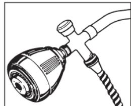
Just a pull on a knob or the turn of a lever and your water diverts where you want it. The shower arm diverter installs easily onto the shower arm with a gasket and plumber tape the shower head installs on to the diverter, again with plumber tape and a gasket. The hand shower unit's hose attaches to the lower outlet of the diverter. Only wall mounted hand shower units will provide a place for mounting the hand shower.
