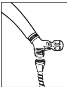
The hose must first attach to a swivel device, which in turn attaches to the hand shower. A swivel is what hooks onto the pin of the mount.
