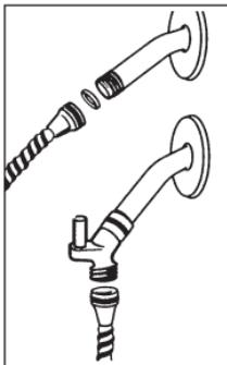
inserted into the hose nut and firmly tighten **CLOCKWISE** onto the water outlet. Do not use a wrench. If your shower comes with a **vacuum breaker** attached to one end of
