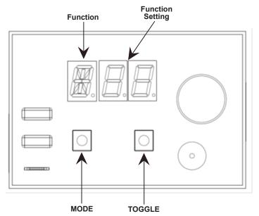
To adjust settings, press and hold MODE (yellow pushbutton on left hand side) until the Function symbol appears. Once in Adjustment Mode, keep pressing MODE until desired Function is reached (see Quick Reference Table). To change Function Setting, press and release TOGGLE (white pushbutton on right hand side) until desired Function Setting is reached (see Quick Reference Table).
