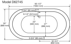
Freestanding tubs use wall-mounted or freestanding faucets. The waste and overflow assembly is concealed between the walls of the tub, eliminating the need for a decorative exposed drain kit.
