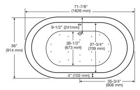
Requires use of a wall-mounted or freestanding tub filler. The drain and overflow assembly is concealed between the walls of the tub, eliminating the need for an exposed drain kit.
