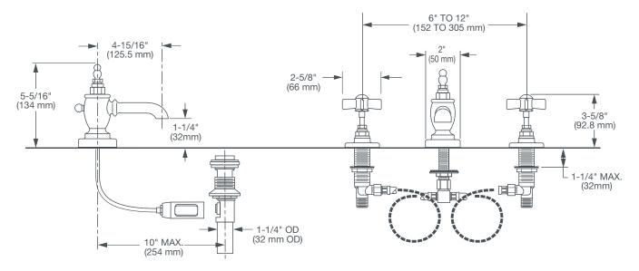
NOTE: MOUNTING HOLES ARE 1-1/4" D. for Spout and for Side valve
