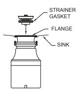
(4) LUBRICATE GASKET ON STRAINER WITH WATER AND PUSH SLOWLY INTO THE FLANGE
