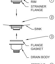
(1) APPLY A SMALL AMOUNT OF NEUTRAL CURE\* SILICONE CAULK / ADHESIVE UNDER THE RIM OF STRAINER FLANGE
