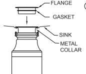
LUBRICATE FLANGE GASKET WITH WATER AND PUSH FLANGE SLOWLY INTO THE METAL COLLAR. PRESS FIRMLY UNTIL IN PLACE.
