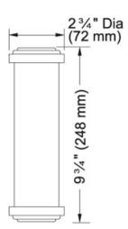
Franke filter cartridges consist of a ceramic outer shell and an enclosed activated carbon block core. Each cartridge utilizes a multistage filtration process to ensure optimal performance. The FRC06 filter cartridge reduces chlorine, particulate & turbidity, cryptosporidium, and lead.
