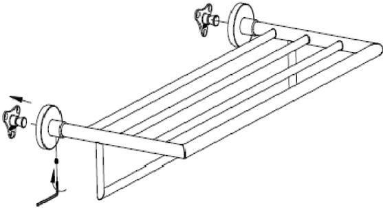
② ALIGN MOUNTING BRACKETS AND MARK LOCATION
