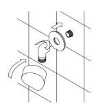
Install the cover over the elbow and snap into place on the gasket. Install the handshower hose.
