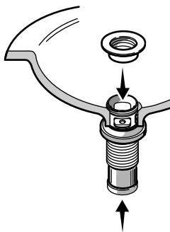
**3** Hold the drain body in place and tighten the nut.
