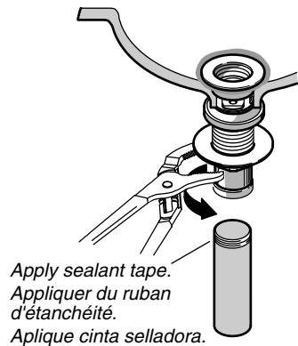
**4** Remove excess putty. Install the stopper. Connect the trap.
