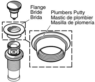
**2** Insert the assembly. Attach the flange.
