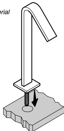
**3** Slide the washer onto the spout shank. Secure with the nut.
