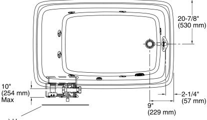
Pump/Control Access 34" (864 mm) W x 15" (381 mm) H
