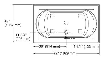
No change in measurements if connected with drain illustrated. (K-7161-AF)
