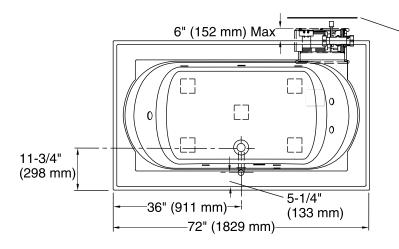
Pump/Control Access 34" (864 mm) W x 15" (381 mm) H
