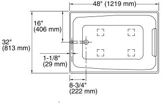
No change in measurement if connected with drain illustrated. (K-7256)
