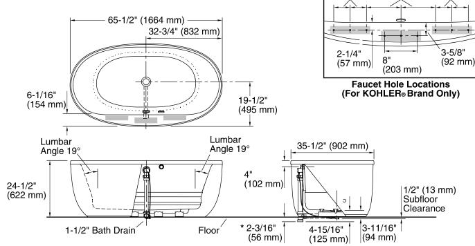
\* Allow for appropriate clearance in subfloor for drain tee clearance. Note: Horizontal PVC pipe and tee shown, not included.
