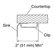
\* Allow clearance around sink rim for clip attachment.
