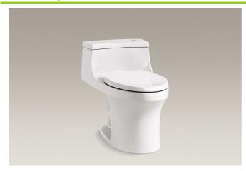
Toilet shall be 27-3/4" (705 mm) in length, 16-3/8" (416 mm) in width, and 25-5/16" (646 mm) in height. Toilet shall be made of vitreous china. Toilet shall be one-piece. Toilet shall feature touchless flush actuation. Toilet shall be a 12" (305 mm) rough-in.
