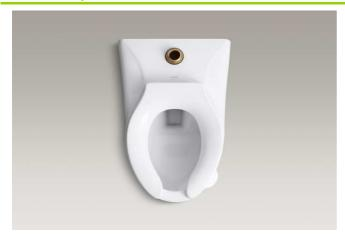
The elongated bowl shall be made of vitreous china. Bowl shall be 26-1/2" (673 mm) in length, 16-1/2" (419 mm) in width, and 13-1/4" (337 mm) in height. The bowl shall be wall-mount with a 1-1/2" top spud. Bowl shall have siphon jet. Bowl shall have bedpan lugs (-L). Bowl shall feature 1.28 gpf (4.8 lpf) or 1.6 gpf (6 lpf) depending on flushometer specified. Bowl shall have 10-1/2" (267 mm) x 9" (229 mm) water area.
