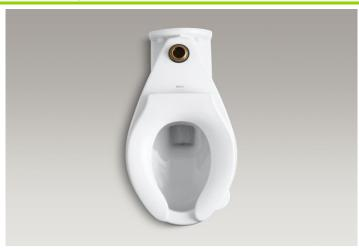
The elongated bowl shall be made of vitreous china. Product shall be 31-1/2" (800 mm) in length, 14-7/8" (378 mm) in width, and 17" (432 mm) in height with a 12" (305 mm) x 10" (254 mm) water area. Product shall be 4" (102 mm) rough-in. Product shall be Comfort Height, less seat and supply. Product shall have 2-1/8" (54 mm) glazed trapway, and a 1-1/2" top spud. Product shall be available with bedpan lugs (-L). Product shall be floor-mount rear outlet flushometer bowl.
