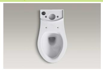
The elongated bowl toilet shall be made of vitreous china. Toilet shall be 28-5/8" (727 mm) in length, 14-3/16" (360 mm) in width, and 32-1/2" (826 mm) in height with 4-1/2" (114 mm) by 5-3/4" (146 mm) water area. Toilet shall be two-bolt installation and 12" (305 mm) rough-in. Toilet shall have 2" (51 mm) glazed trapway. Toilet shall be 1.6 gpf (6.0 lpf) or 1.0 gpf (3.8 lpf) with dual flush flushing system. Toilet shall include polished chrome push buttons and supply line.
