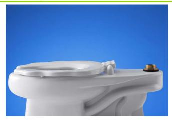
The elongated toilet bowl shall be made of vitreous china. Bowl shall be 26-7/8" (683 mm) in length, 12-7/8" (327 mm) in width, and 12" (305 mm) in height with a 12-3/8" (314 mm) by 10-1/8" (257 mm) water area. Bowl shall be 10" (254 mm) rough-in with a 1-1/2" top spud. Bowl shall be 1.28 gpf (4.8 lpf). Bowl shall include K-4686 toilet seat with scalloped handhold locations for children. Bowl shall have a choice of white, primary yellow, primary red, or primary blue colored seat.
